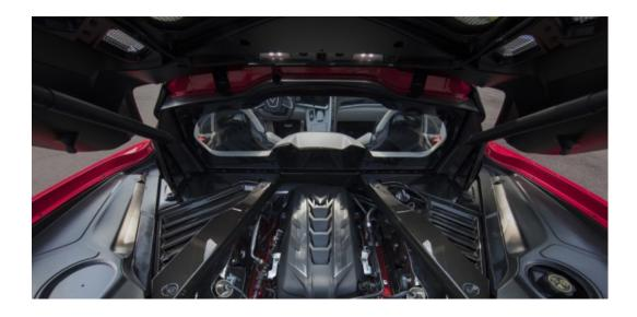
C8 Corvette customers should exercise caution when using a pressure washer under the hood, keeping the nozzle at least a foot away from all surfaces, as well as keeping the nozzle at a 40-degree wide angle spray pattern, or wider. Finally, owners should pay attention to any components under the hood that have a symbol indicating that they should not be pressure washed, as seen below:
