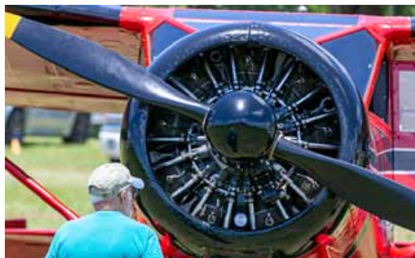
An aviation enthusiast checks out the large 9 cylinder radial engine of a 1944 Stinson
